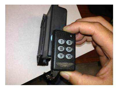
Hold the remote in this position for 10 seconds. The unit will emit a beep and now be in remote programming mode. Press button 1 on the TX and the unit will beep to confirm. Repeat this step for additional TX. Up to 4 TX can be learned to the unit. After all TX have been learned the unit will exit programming after 10 seconds and emit a beep to confirm it has exited.
