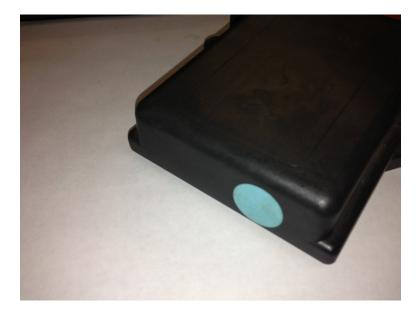
There are magnets located inside the back cover of the remote and a reed switch in the controller that the magnet will activate if placed in the proper position.
